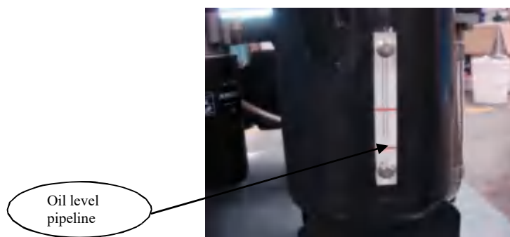
Picture 10.1 The oil level should be kept between the upper and lower red lines of the oil mark
